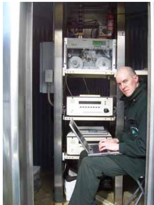
Monitoring officer, Karl Watson, calibrates a carbon monoxide analyser inside the Wellington central monitoring station
