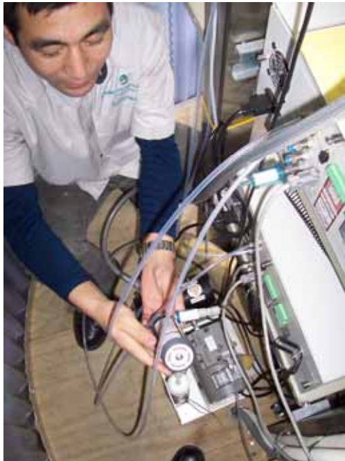
Senior monitoring officer, Darren Li, carries out maintenance on a nitrogen dioxide analyser at the Wellington central monitoring station
