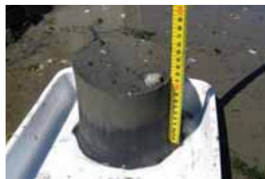
Measuring the depth of oxygenated sediment in a sediment core sample from the Porirua Harbour. The greater the depth of oxygenated sediment, the better the conditions for plant and animal life in the sediment.
