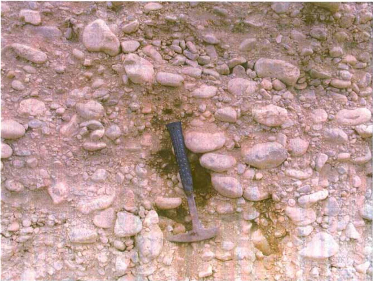
Figure 7. Typical in-situ profile of gravel, cobbles and sand forming cut slope in old excavation.
