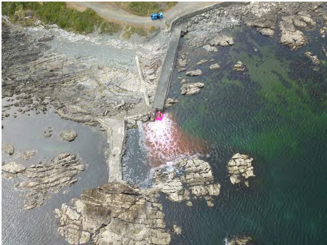
Figure A.1 Drone image of the dye test as the dye emerges from the outfall at 10:30 on the 29 th November 2017.
