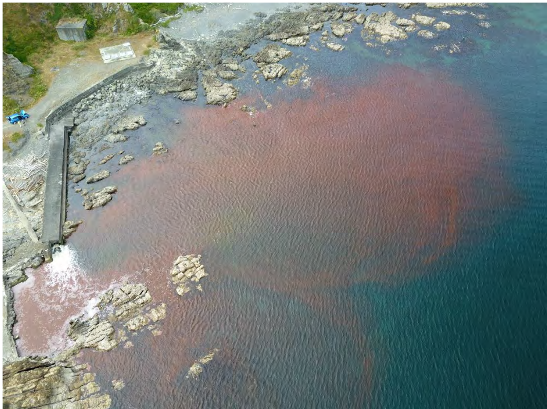
Figure A.9 Drone image of the dye test at 10:38 on the 29 th November 2017.
