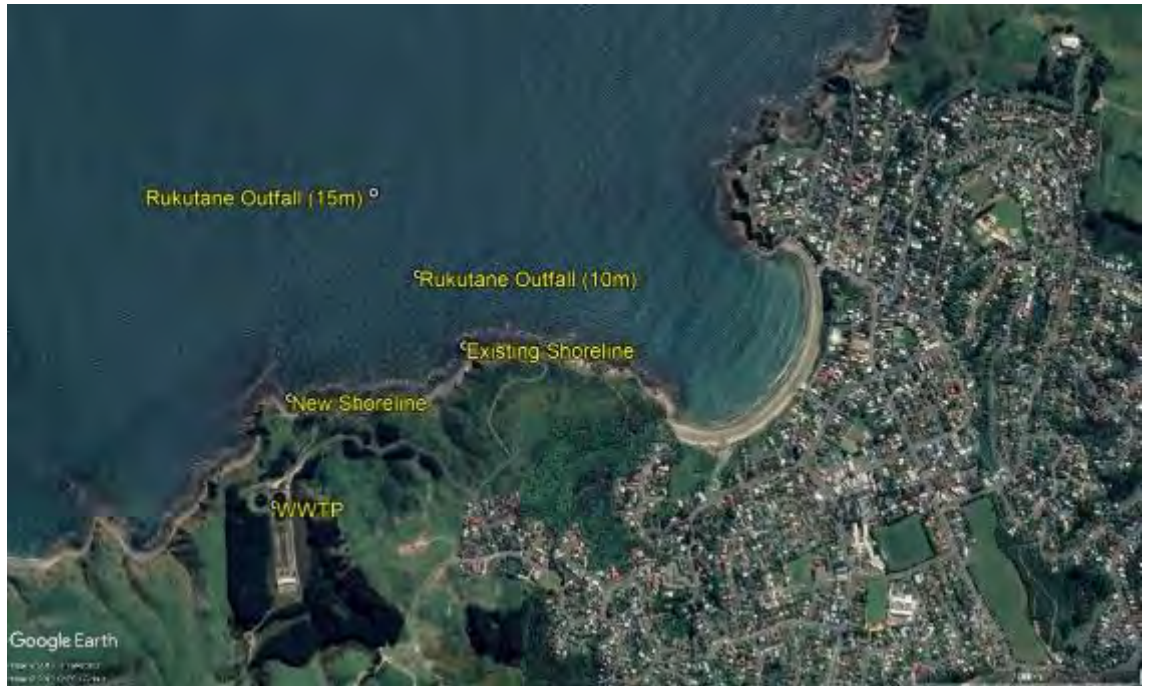
Figure 2-1. Location of existing shoreline discharge, offshore outfalls and new shoreline discharge at Round Point.
