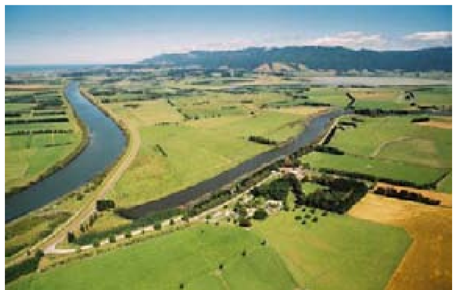
The Ruamahanga River diversion has made thousands of hectares of land available for farming. However, because it is still susceptible to occasional flooding, the area is not suited to more intensive development.
