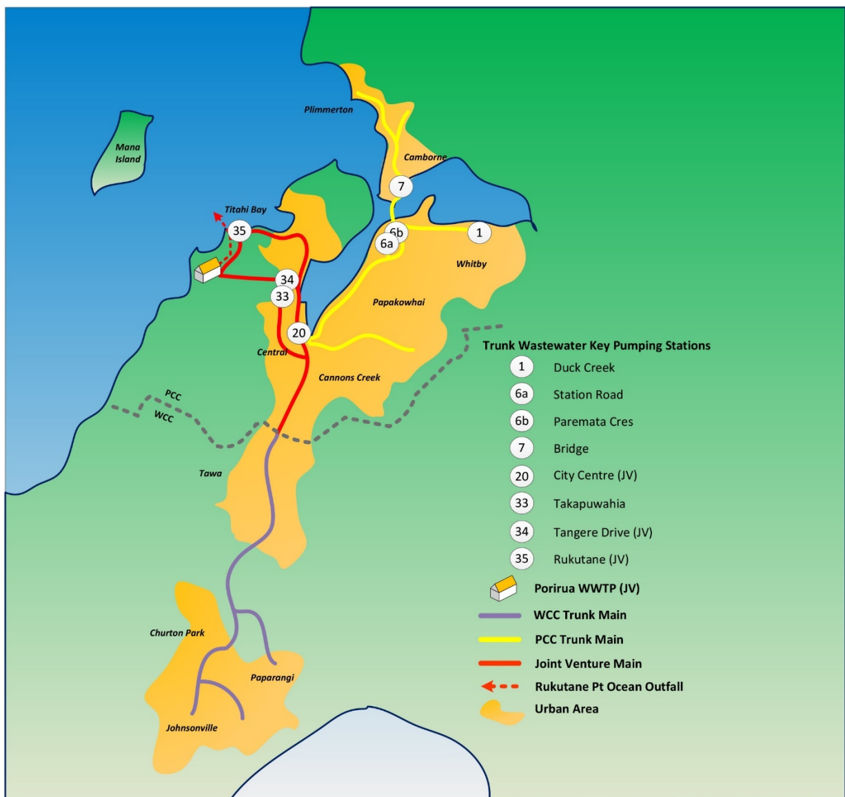
Figure 1-1: Overview of the Porirua wastewater system
