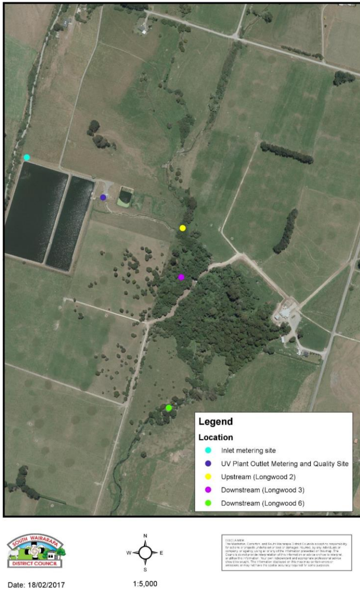
Figure 1: Indicative WWTP flow and water quality monitoring site locations
