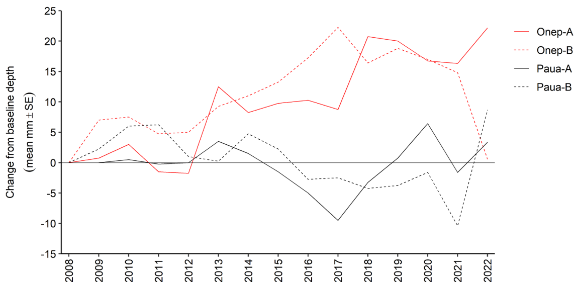
Fig. 4. Mean change ( \pm SE) in sediment depth over buried plates since the baseline was established in 2008.
