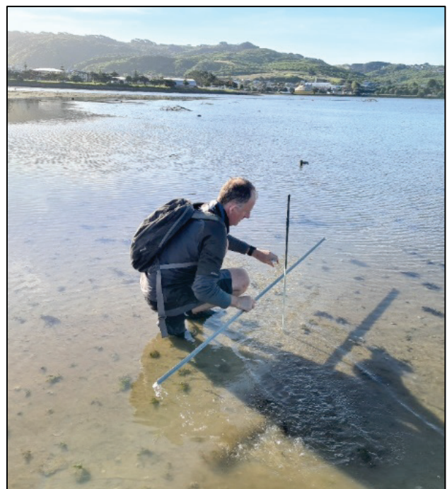
Measuring sediment plates at Paua A in the Pāuatahanui Inlet
