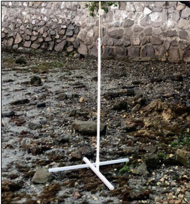
Custom-built subtidal measuring frame
