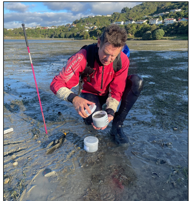
Collecting sediment samples for laboratory analysis, Browns Bay intertidal Site P11, Pāuatahanui Inlet.
