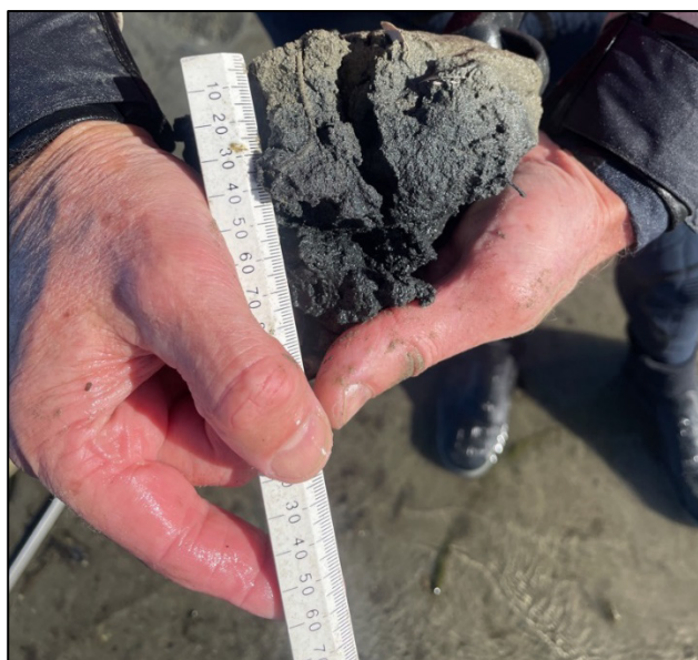
25mm of oxygenated sand above organically enriched sediment Por B (O3), Onepoto Inlet.
