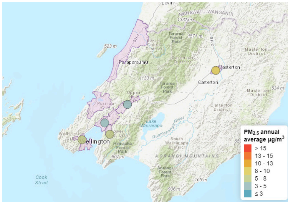
Figure 6: Annual PM 2.5 summary results are shown in the map and table. Annual averages are only reported for sites with more than 75% data capture.
