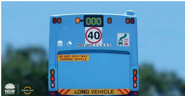
Figure 6.7 Flashing ‘wig wag’ lights and signage on a New South Wales school bus (reprinted from New South Wales Government, 2022b)
