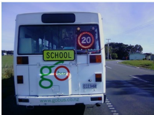
Figure 6.5 Flashing LED '20' roundel sign on a school bus, as part of the 2011 trial (reprinted from Transport Engineering Research New Zealand, 2011, p. 13)
